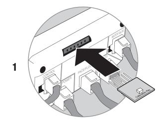
Insert Calibration Key as shown (LED side up) into 6-pin connection in ECU
